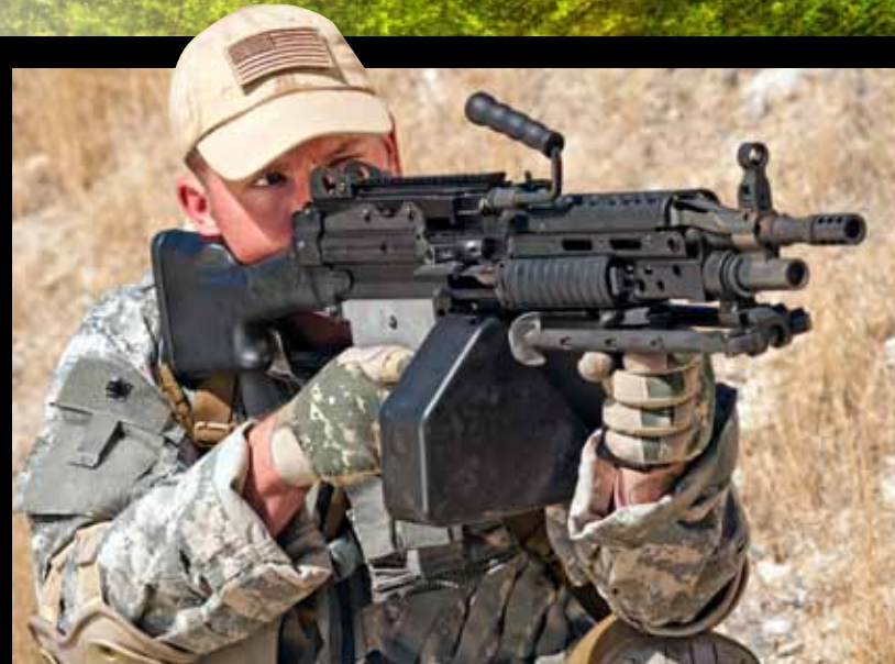
Although originally designed to be used primarily from a prone position, the MK46 and its other configurations can be shoulder-fired with ease. For a light machine gun, recoil is noticeably lighter and the weapon is easy to keep on target with help from a vertical foregrip.
