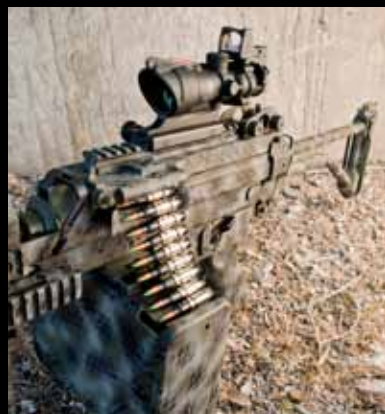
MGA's lighter and more portable MK46 configuration feeds from a reliable 200-round box mag, which provides a significant advantage on the battlefield or emergency SWAT situation.
